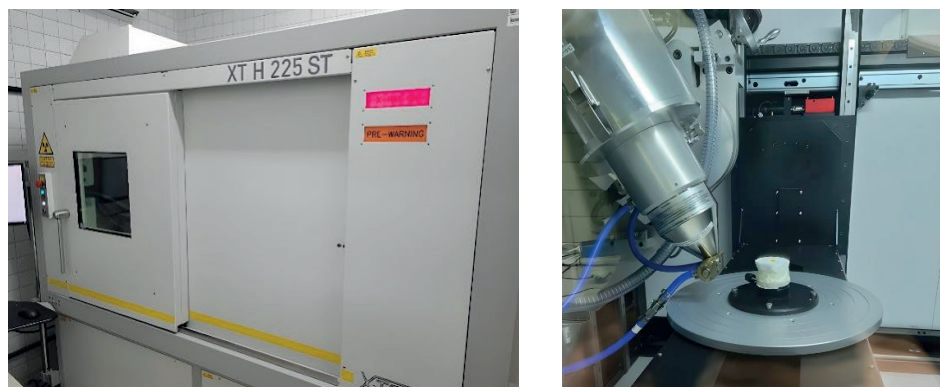
Figure 10: Left: Industrial CT Scanning - XT H 225 ST. Right: Internal view of XT H 225 ST with Citrus sample. Source: developed by the authors in collaboration with DEN.
