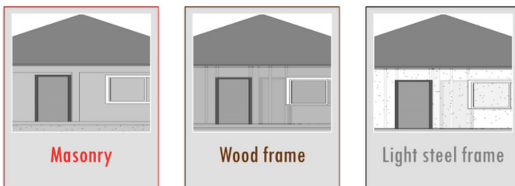
Figure 10: Building in three construction methods
