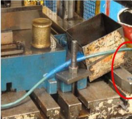
Figure 8. Inadequate fixing screw.
